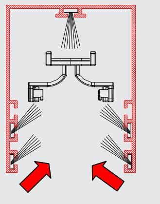
**1** PLACE THE TOP TRACK (A). AFTER HAVING MARKED AND DRILLED, FIX IT WITH THE SUPPLIED SCREWS.
