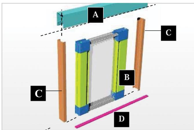
BRUSH PILE SHALL BE SET UP WITH BRISTLES UPWARDS.
