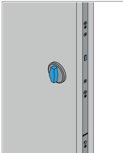
► Mount the fittings for the safety lock T2 according to the enclosed assembly instructions of the producer.
