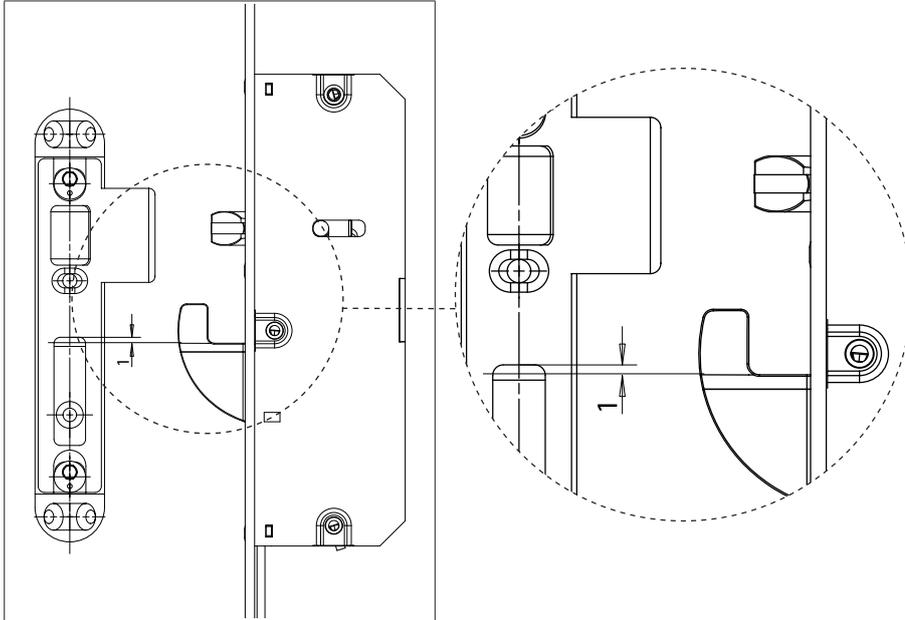
The hook bolt must not exceed an interval of 1 mm from the frame part.
