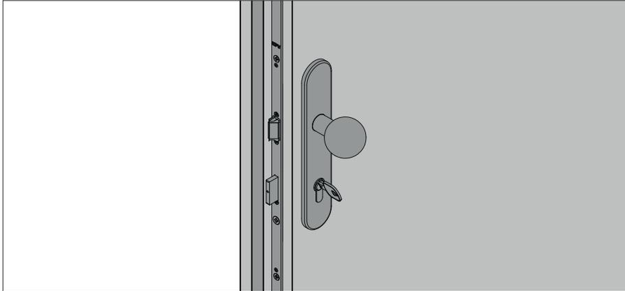
► Mount the fittings for the main lock according to the instructions of the producer.
