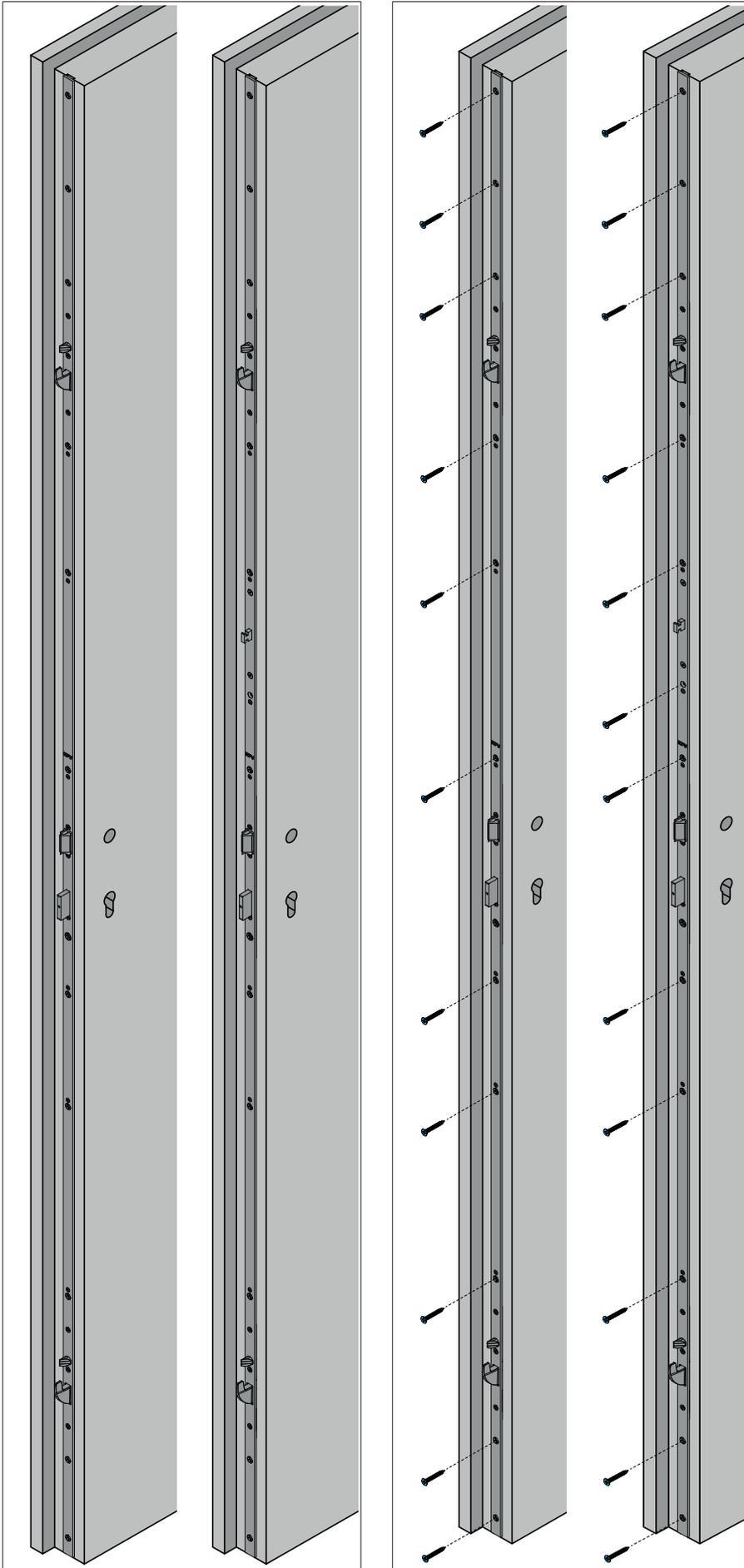
► Screw the multi-point lock onto the door leaf:
